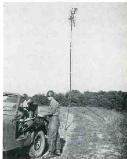
This Signal Corps "radar ruler," used for great distances, enables a surveyor to survey 50 miles at a time accurately and in any weather.
