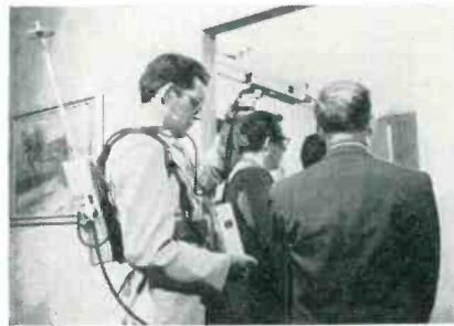
Fig. 1: Operating test of RCA experimental portable TV camera and back-pack transmitter. Electronic viewer is in operator's right hand. Tiny unit in other hand is Vidicon camera unit.
