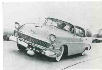
Bomb-shaped TV camera is on front of car, under bumper, for quick engineering observation in auto research.
