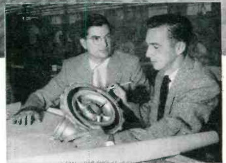
AiResearch two stage lightweight gas turbine compressor provides pneumatic power for aircraft main engine starting and serves as auxiliary power source for a variety of ground and in-flight services.
